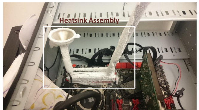
Figure 5: Setup-B utilizes the host machine with CCH assembly mounted on DDR4 DIMM. Memtest86 is used to characterize the DIMMs.
