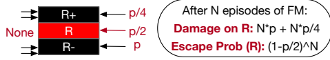
Fig. 15. Attack R by maximizing ACTs on R+ and R- while no ACT on R .
