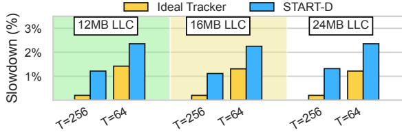
Fig. 9: Impact on slowdown as LLC size is varied. START-D performs similar to ideal tracker at different cache sizes.
